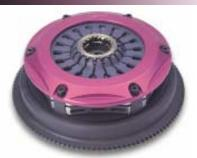
For high-powered applications, EXEDY offers twin and triple Multi-Plate Clutches. These are designed for hot street action as well as drag, road and rally racing. The twin plate clutches are rated for above 500hp to 750hp. The triple plate clutches are rated for up to and over 1000hp (for drag race applications). Multi Plate clutches include a billet chromemoly steel flywheel.
