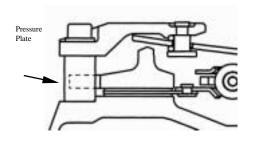
The diaphragm sping clamp load is relieved and pressure plate is free. But, the pressure plate does not clearly sperate from the disc due to friction at the lug.
