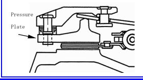
With a strap drive system, the pressure plate is lifted by the force of the straps.
