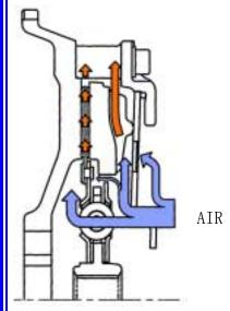
With the EXEDY turbine type pressure plate, the temperature is maintained equally on the pressure plate side and the flywheel side, reducing distortion and improving facing life.
