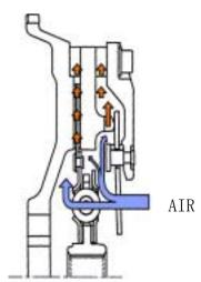
In a normal clutch, the pressure plate has less heat capacity than the flywheel, therefore tends to run hotter. This causes distortion of the disc facings.
